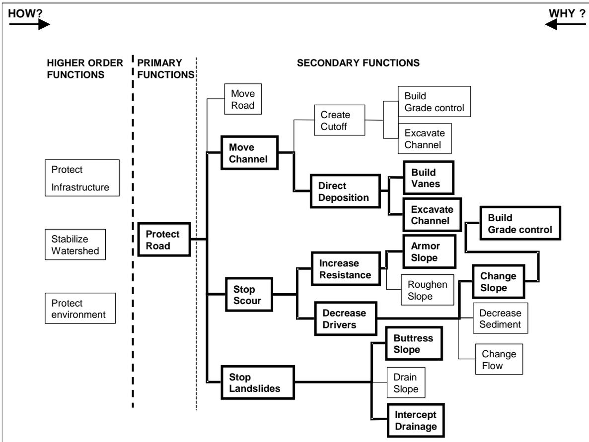
Figure 4. FAST diagram, Strecker Road Protection
