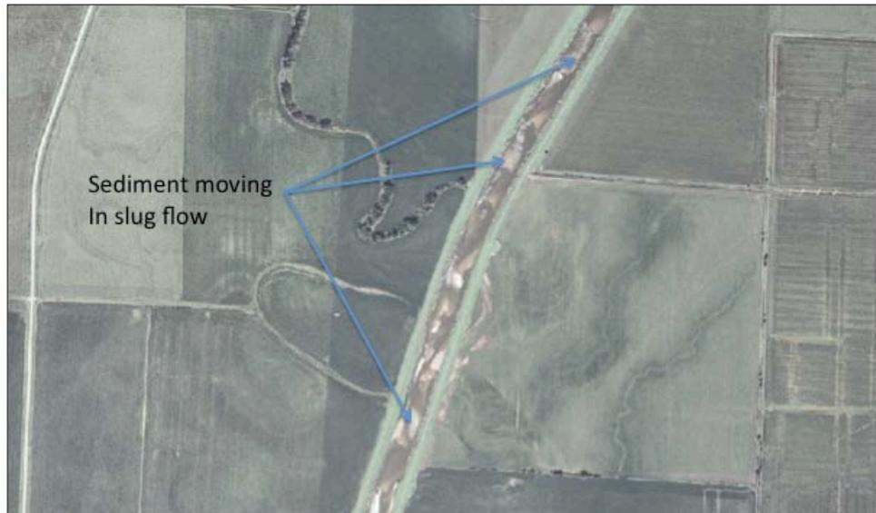
Figure 3. Sediment released from upstream berms accumulating in downstream reaches (from NRCS geodatabase)
